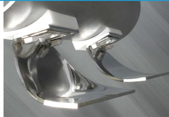
Close-up of the Triosim pulp washing shower section shows Orifices, lock plates, and the new radiused Deflectors Lips.
