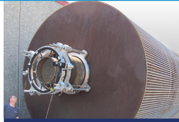
Triosim's Project Manager, checks the settings on the portable lathe that will be used to rebuild the washer drum trunnion. Although this project was completed off-site, one of the most important design advantages of the portable lathe is its ability to machine trunnions without removing the washer drum from the vat.
