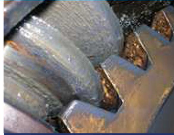
Gears above have been eroded by water contamination of the gearcase.
