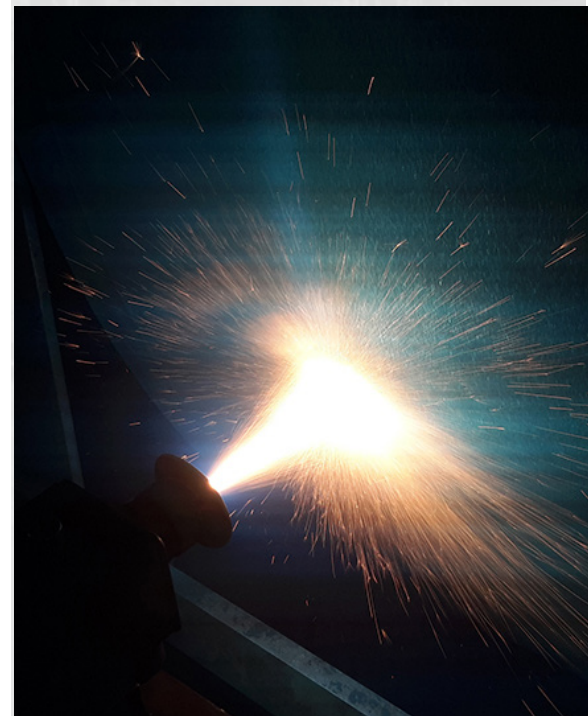
95" drum being coated with 420 stainless steel.
