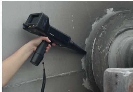
*Triosim technician checks for a leak in a washer drum using Ultrasonic technology.*
