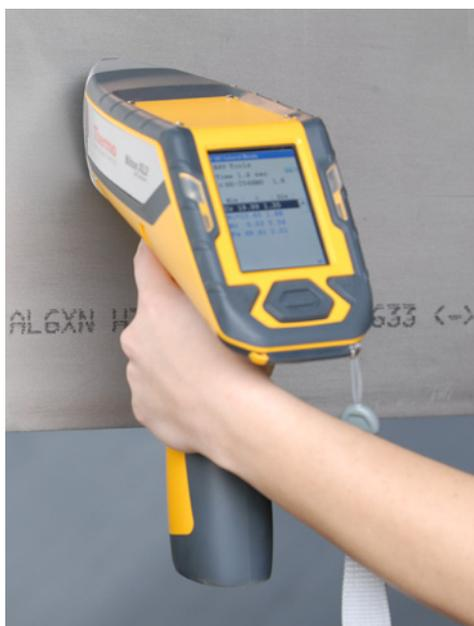
*Triosim Technician performs a material analysis on a sheet of 6% moly stainless steel. Confirmation of material is critical, as it will be used in the bleach process, where any lower grades of metal will disintegrate.*
