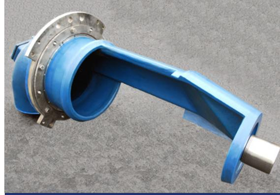
This FRP Discharge Valve was remanufactured after a decade of service in an extremely aggressive environment. Expected service life is similar to that of a new valve while the cost was less than around half of a new one.
