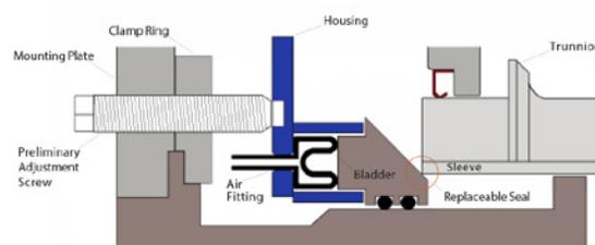
The DF-II uses air (low psi), to provide a uniform application of pressure around the entire circumference of the seal. This pressure is applied as the air bladder (see illustration, below) fills with air. This avoids the uneven pressure along the sealing surface that can result from manual adjustment of the pressure.
